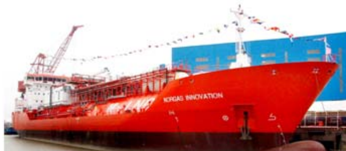
Norgas Innovation – 1 st Multigas vessel Naming Ceremony. The ship is an advanced LNG/ LPG/ Eth gas carrier – 10 000 cbm.
