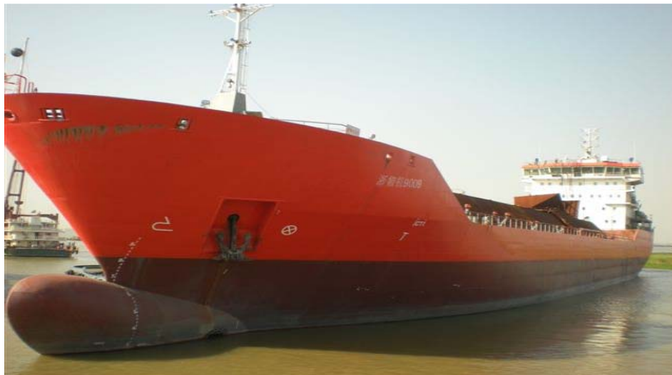
The Norgas Innovation – the first Multigas-vessel of a series of 6 and under outfitting stage as being completed by Skaugen Marine Construction in China (SMC). The ship is an advanced LNG/ LPG/ Eth gas carrier – 10 000 cbm
