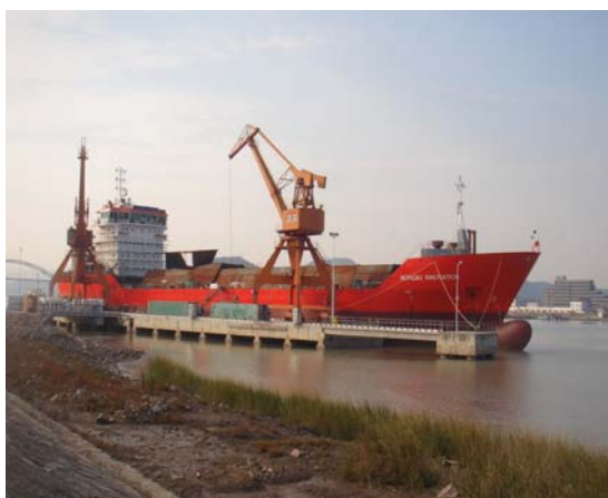
Norgas Innovation (MG#1) berthed for the outfitting stage of the shipbuilding process
